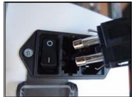
**Fig. 20: Replacement of fuses**
