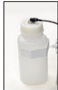
Fig. 5: Check of condensate collection vessel
