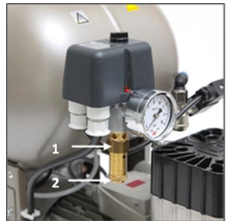
Fig. 7: Check of safety valve
