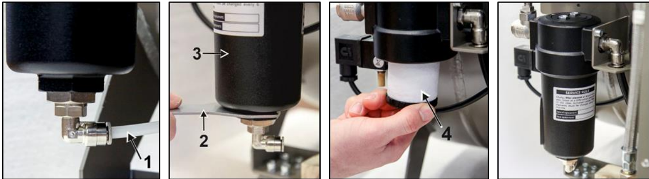
Fig. 19: Filter element replacement
