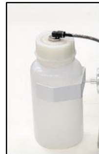
Fig. 16: Check of the condensate collection vessel
