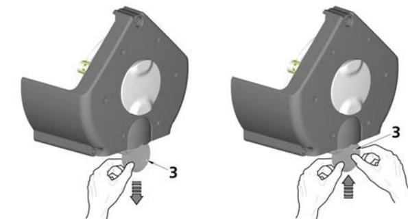
Fig. 18: Inlet filter replacement
