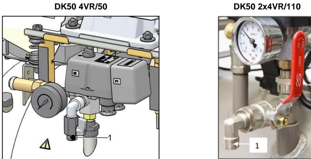
Fig. 8: Connecting to the compressed air outlet
