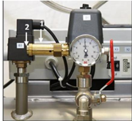
Fig. 17: Check of safety valve
