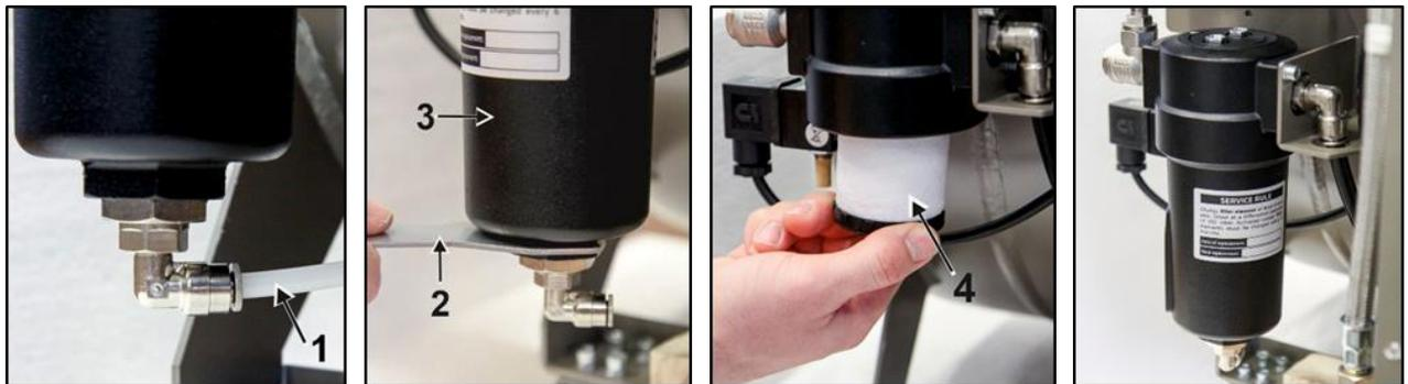
**Fig. 19: Filter element replacement**
