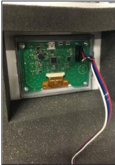
Fig. 17: Connecting the display connector
