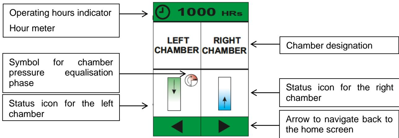
The dryer operating hours indicator is located at the top of the screen. The dryer operation screen is also divided into 4 sections, which describe the dryer chamber working cycles using a graphical depiction of the operating states of each chamber.
