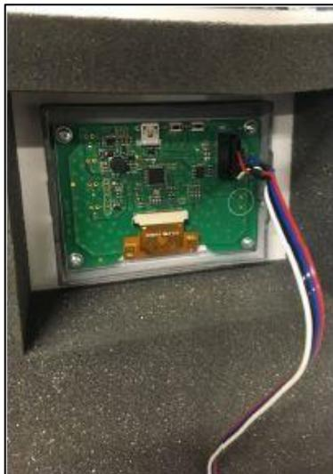
**Fig. 17: Connecting the display connector**
