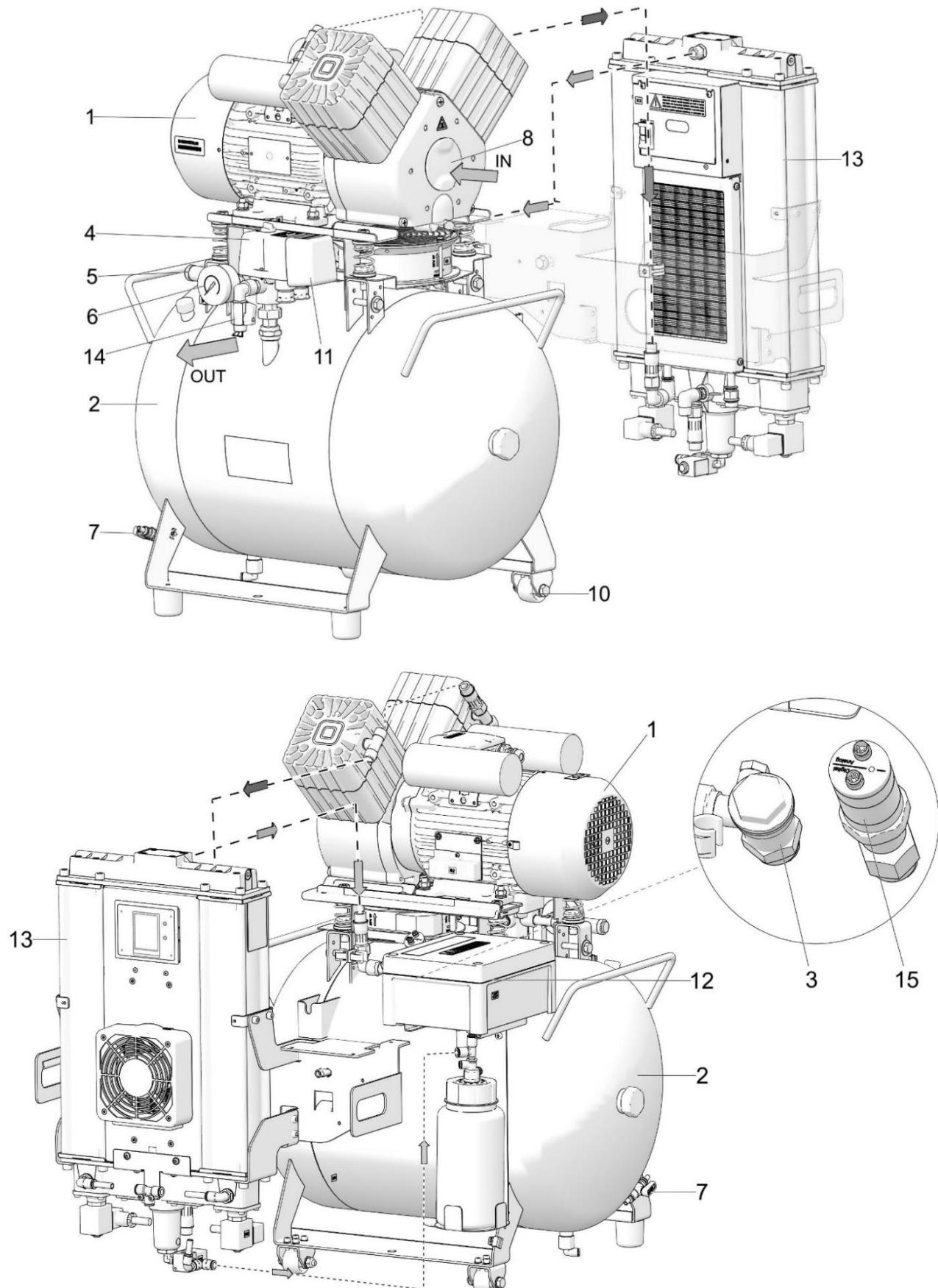
**Abb. 2: DK50 2x2V/110/M – Kompressor mit Adsorptionstrockner**
