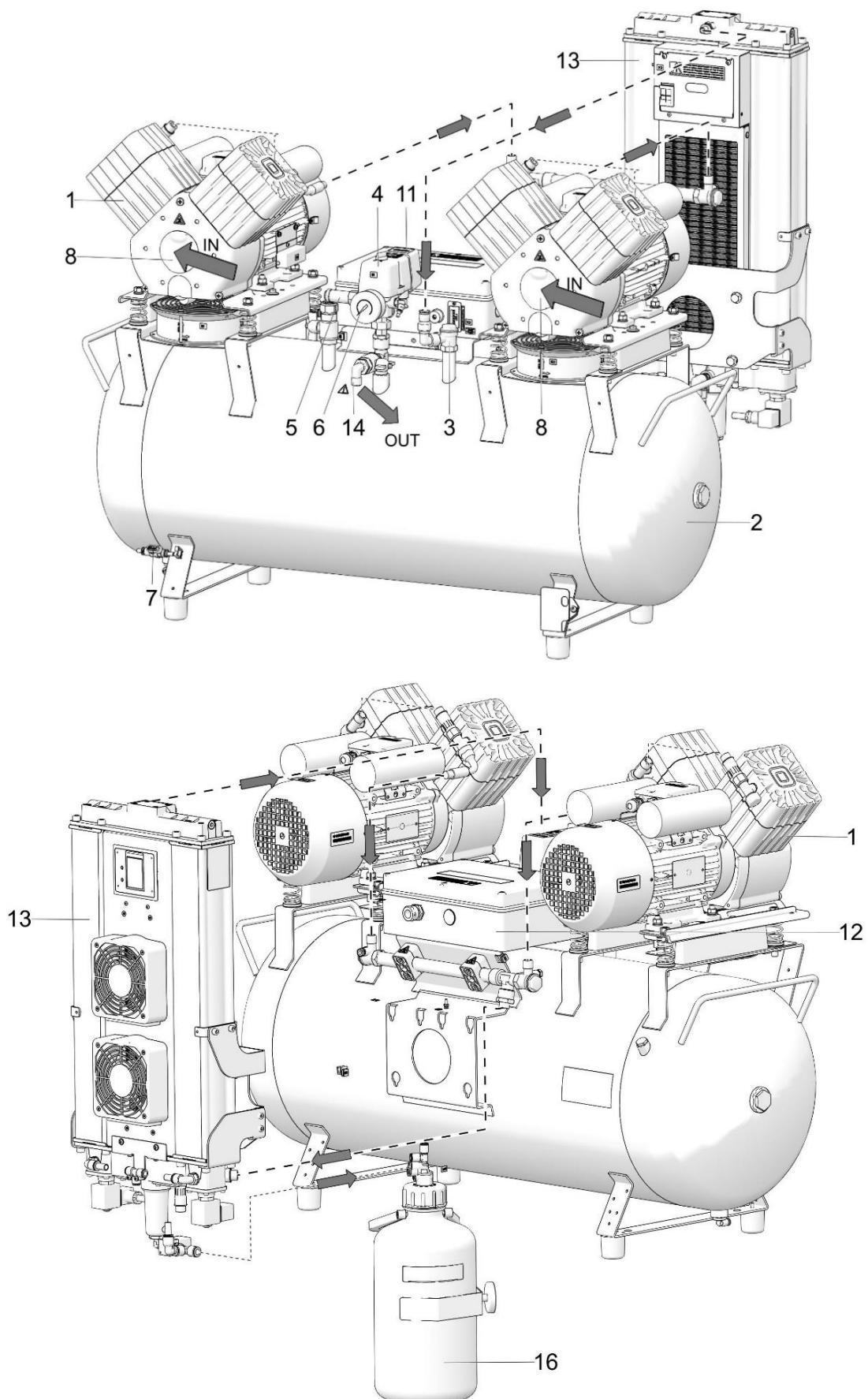
**Fig. 3: Adsorption dryer**
