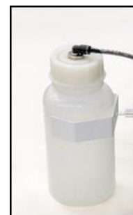
Fig. 15: Check of condensate collection vessel
