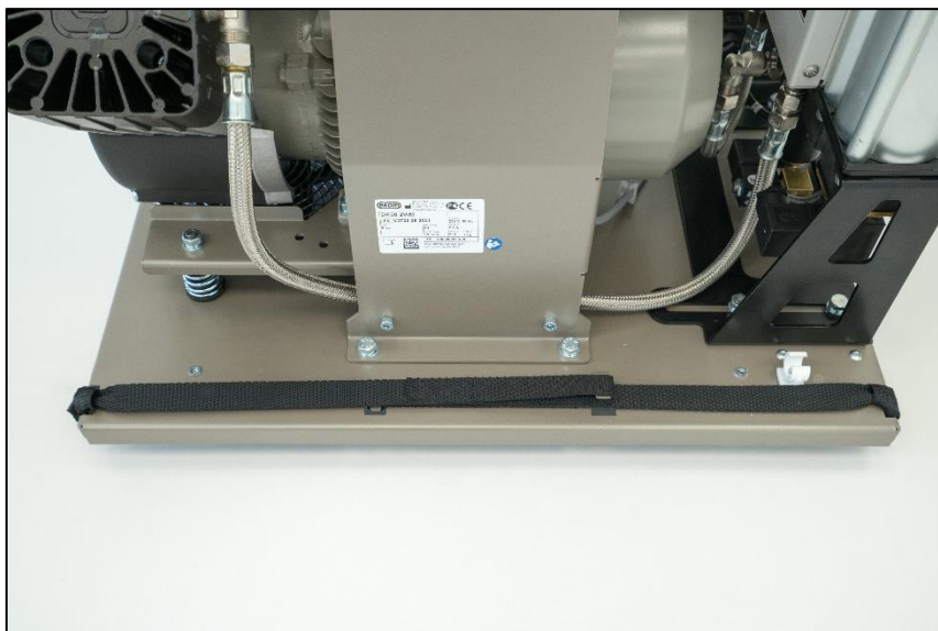
Securing of handling straps after putting compressor at the place of operation
