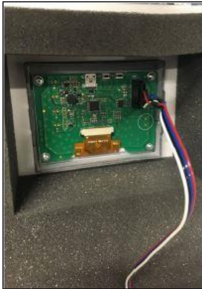
Fig. 15: Connecting the display connector
