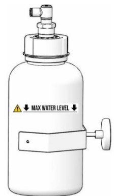
Fig. 18: Check of condensate collection vessel
