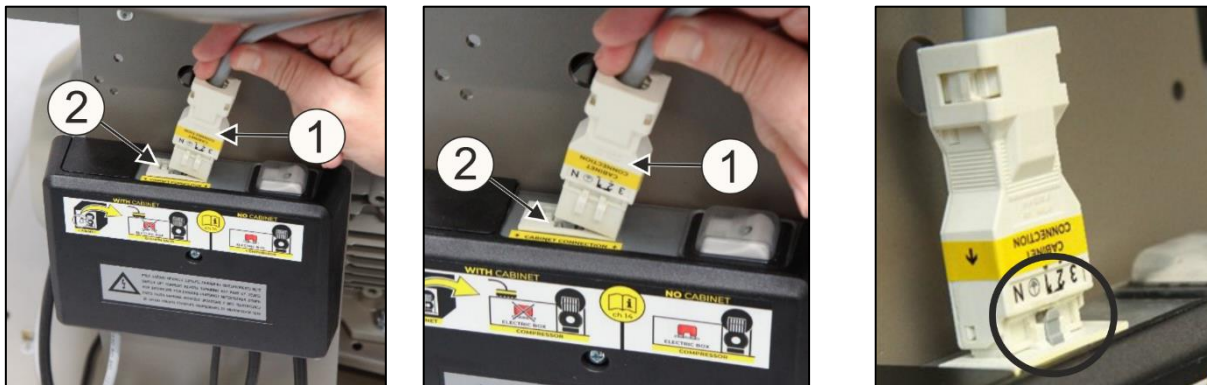
Fig. 11: Connecting a compressor installed in a cabinet
