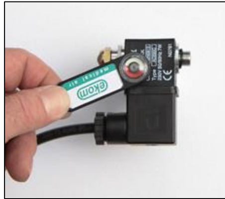
Fig. 19: Check of solenoid valve operation
