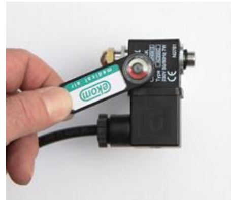
Fig. 24: Check of solenoid valve operation
