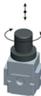
Fig. 15: Setting outlet air pressure
