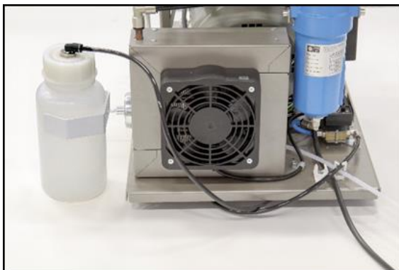
Fig. 7: Connection of condensate collection vessel
