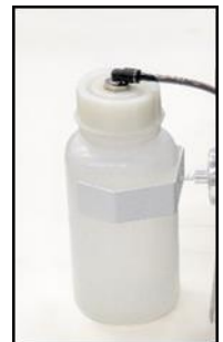
Fig. 11: Check of condensate collection vessel
