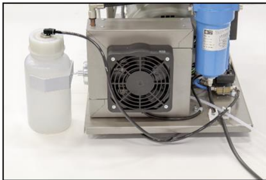
Fig. 7: Connection of condensate collection vessel
