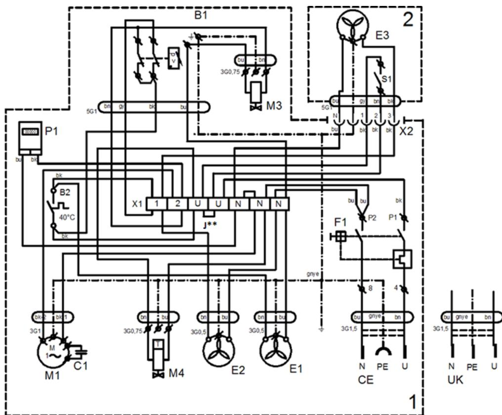
J\*\* - Connect the jumper only for compressor models not installed in
