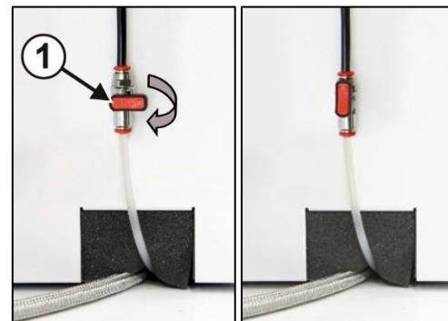
**Fig. 10: Condensate drain from the pressure tank**
