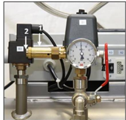
Fig. 17: Check of safety valve
