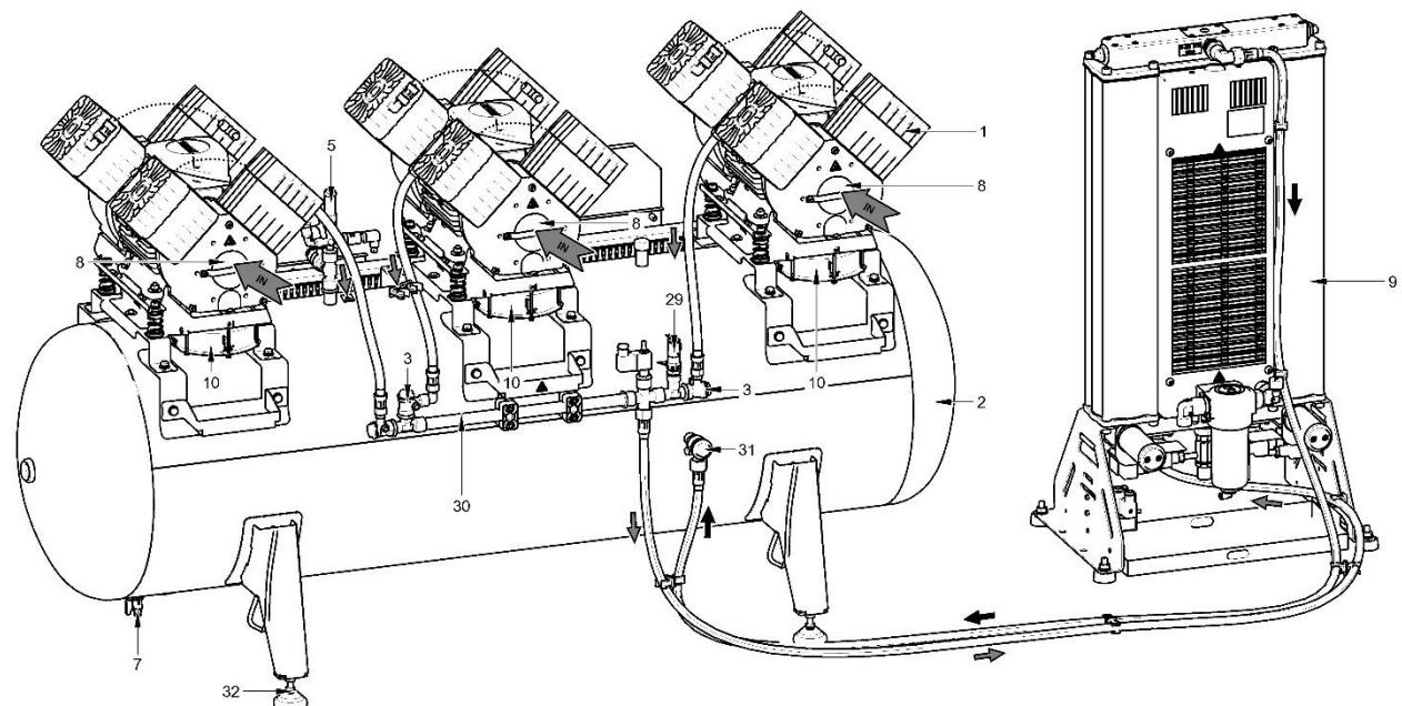
**Рис. 2: Адсорбционный осушитель**
