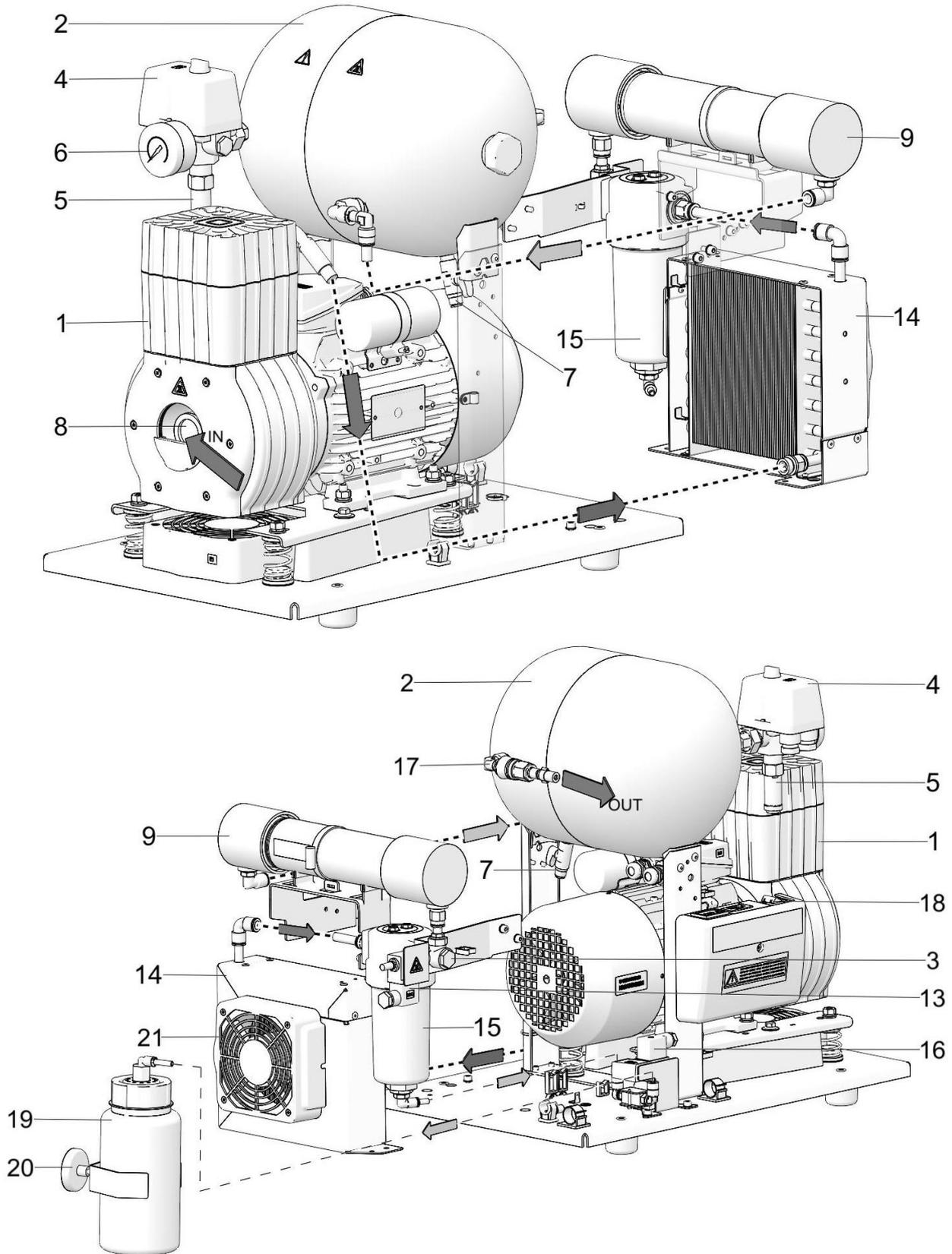
Fig. 3: Compressor DK50-10 S/M (8-10bar)
