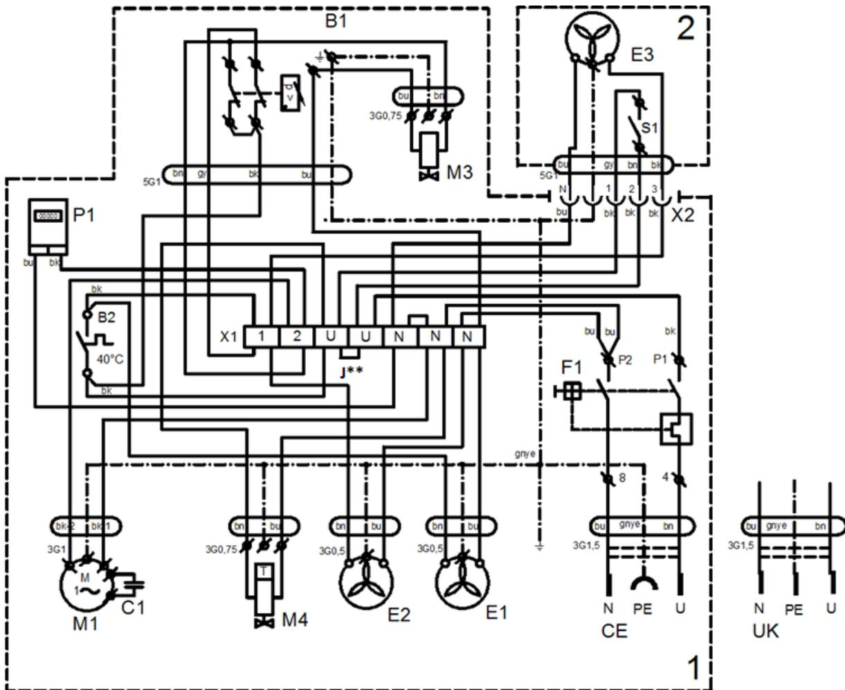
J\*\* - Connect the jumper only for compressor models not installed in cabinets (chap.19.10)
